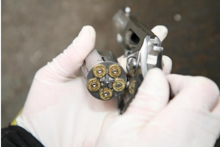
Four expended cartridge casings and one live round inside the chambers of the revolver's cylinder.
