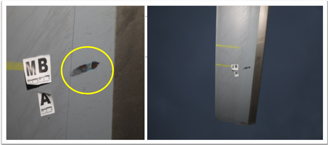
Figure 4: Images of the shotshell strike on the rotor of the LASD helicopter.
