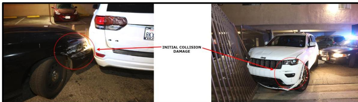
**Figure 2:** Photograph shows front end damage to vehicles from the Jeep ramming the patrol car.
