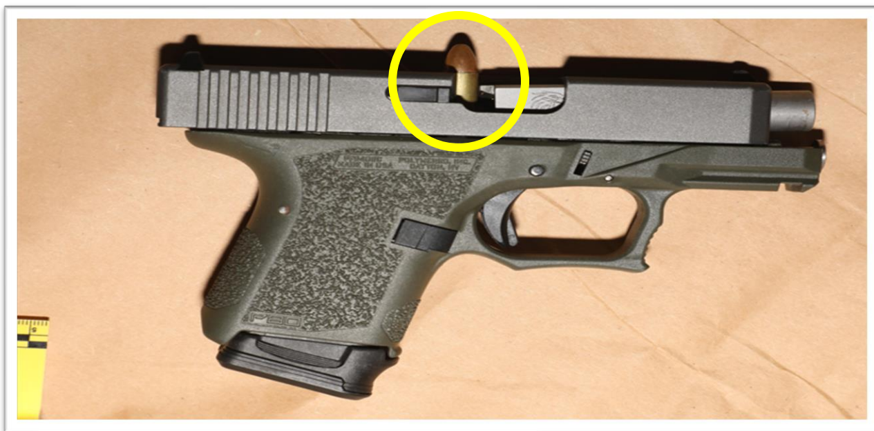
Figure 2: Salazar's Polymer 80, model 940SC, with the misfired round, circled in yellow.
