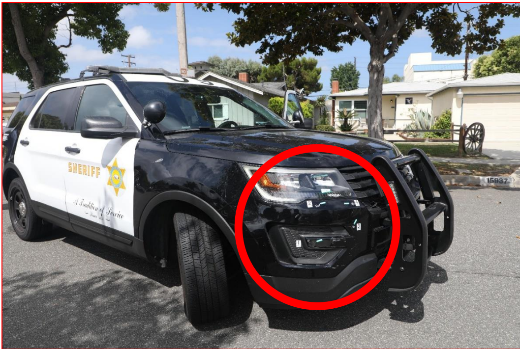
Figure 3- Photo of Damage to the Right Front Bumper of the Patrol Vehicle.
