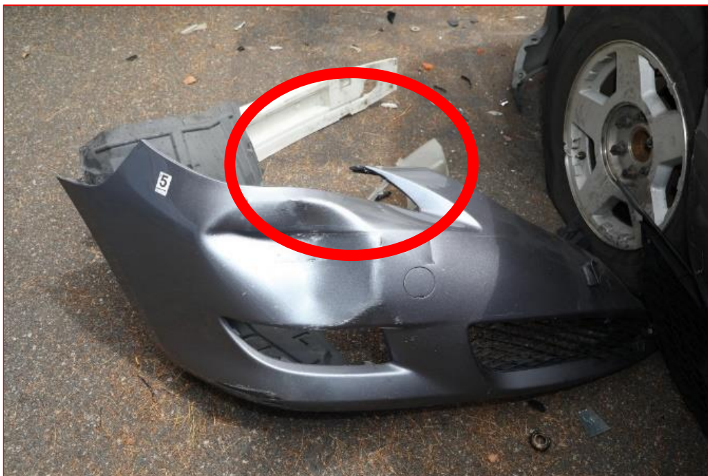
Figure 4- Photo of damage to the Right Front Bumper of Hudson's Mazda.
