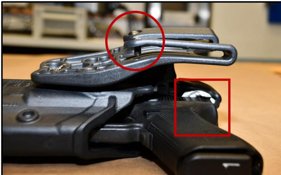
The photograph depicts Mosely's handgun before it was removed from the holster. The belt loops of the holster (circled) were unsecure due to broken rivets. The paper beneath the hood of the holster (boxed) is also pictured.
