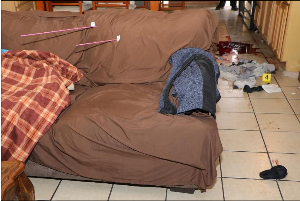
Figure 8 – LASD picture shows two bullet impacts in the couch marked with trajectory rods. The left rod marks the round that stopped in the couch frame. The right rod marks the round that exited the couch.
