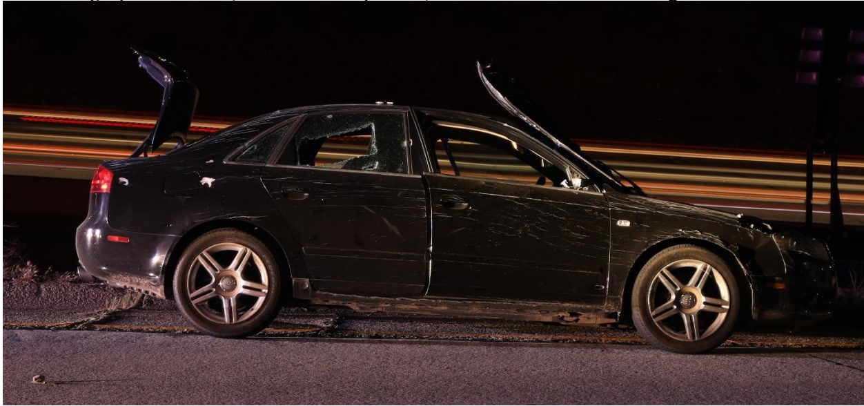
Photograph 6 - Audi (at terminus of pursuit) with hood bent back flat against windshield.
