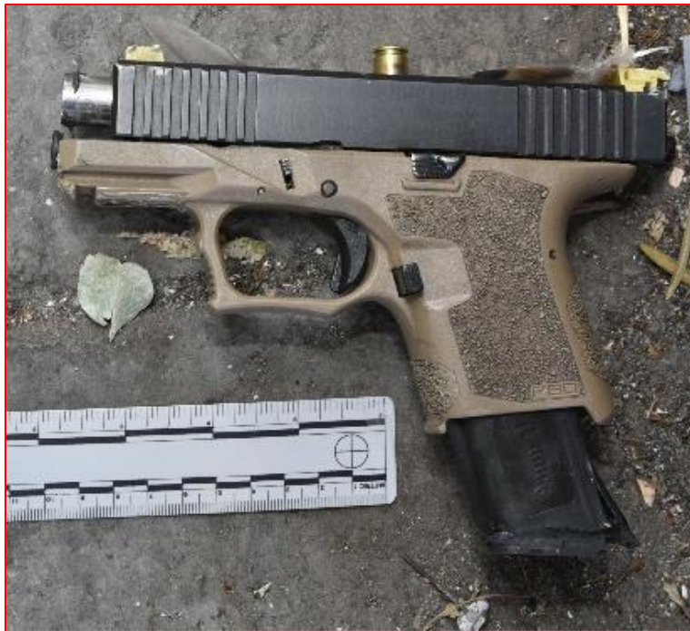
Figure 4- Photo of James' Gun with “Stovepiped” Casing.
