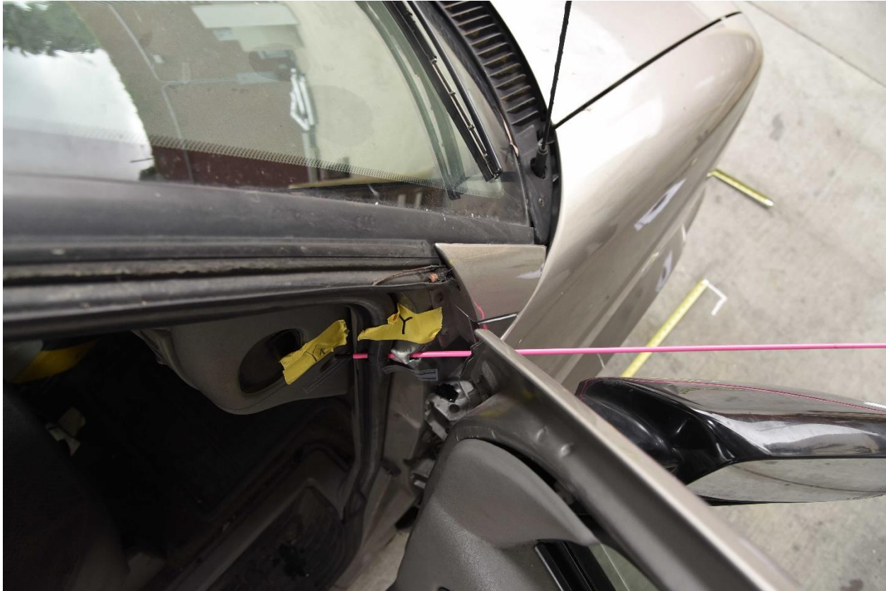
Photograph 2 - Bullet impact and path into interior of front passenger compartment.
