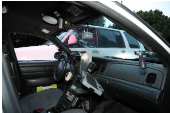
Figure 4: Darringer's car was equipped with electronics which partially blocked his egress.
