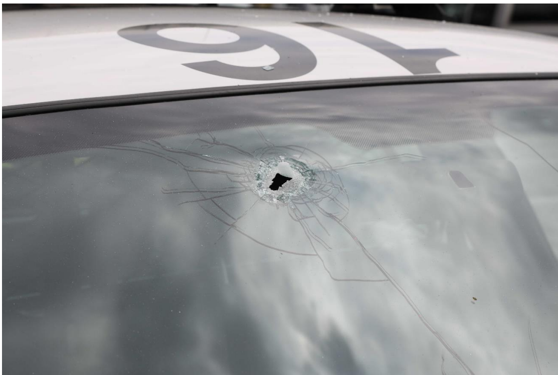
Close up of the bullet impact to the top of Unit 820's windshield.
