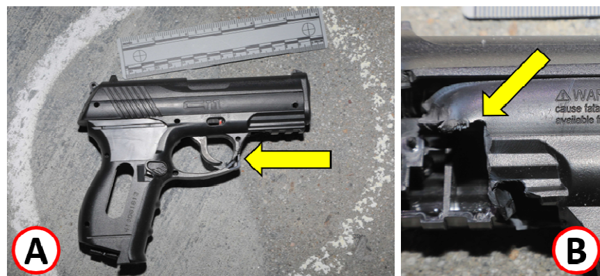
Figure 4: Air pistol held by Brown during officer-involved shooting. (A) depicts right side of air pistol; (B) depicts left side of muzzle. Yellow arrows indicate damage from shot from Lopez' shotgun.
